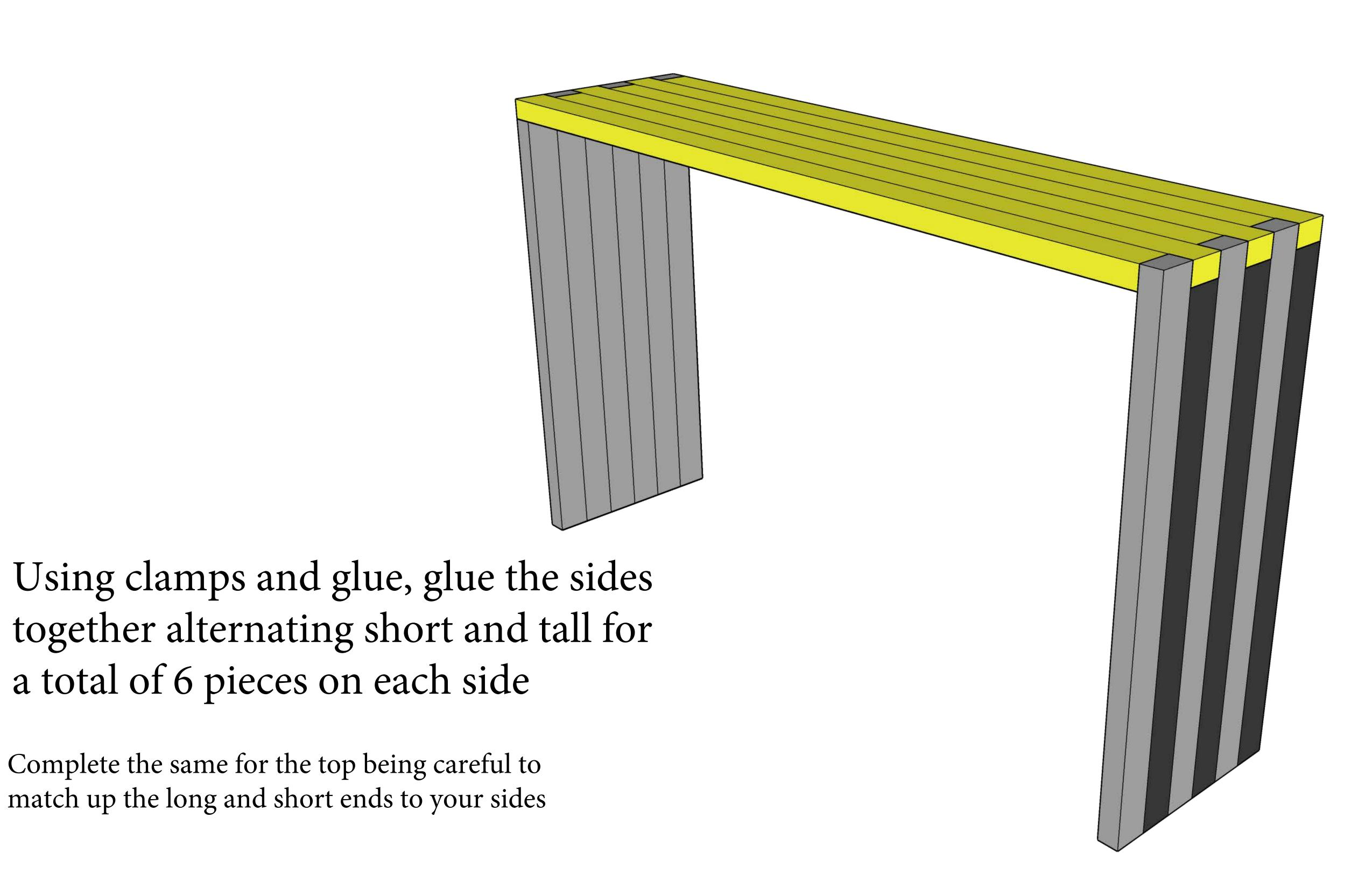
Attach the top to the sides with glue and clamps clamping the entire width of the table.
